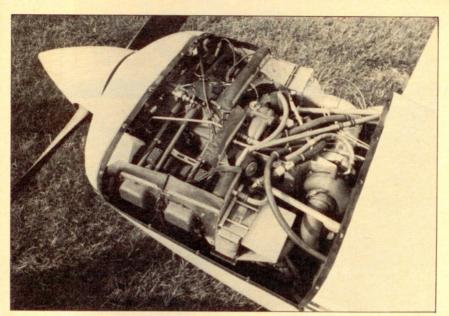
You rarely get something for nothing, and turbocharging is no exception. Look at all that hose and ducting! TBO for the Lycoming TO-360 is 1,800 hours—200 hours less than the normally-aspirated Seminole, mainly because of higher operating temperatures associated with turbocharging. The airplane pictured in this article is one of the first Turbo Seminoles and does not have the new landing lights.
