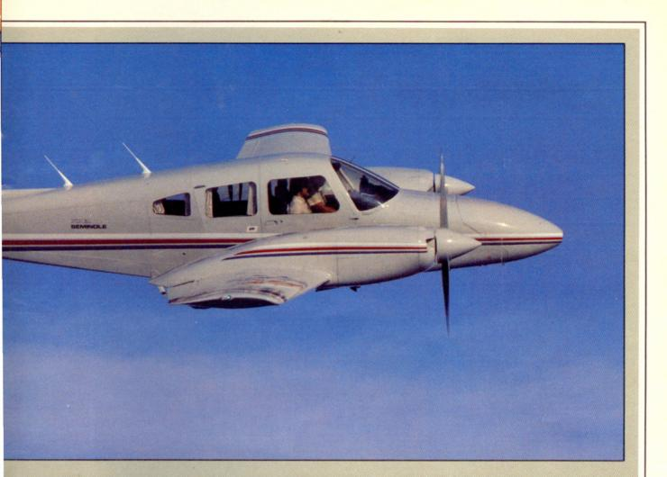
tennas have an unobstructed "view" of the weather ahead. The post-October Turbo Seminoles have two landing lights mounted on the underside of the nose section, and inlet air comes from a NASA-type flush air scoop on the left side of the nose. The only other things that distinguish a Turbo Seminole from the standard model are the louvers on top of the engine nacelles and single, rather than double, exhaust pipes. And, of course, the new paint schemes.
